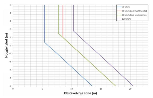
**Figure 18** – Effects of the ascending and descending slopes to the size of the standard obstacle-free zone (Dutch Ministry of Infrastructure and the Environment, 2017)
