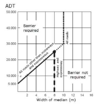
**Figure 20 –** The Parameters Which Determine the Installation of Barriers in the Median (Ministry of Infrastructure and Spatial Planning, 2013a)
